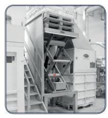
Lifting tables in mixed materials can be made e.g. galvanized scissor and bottom frame and stainless steel platform.
