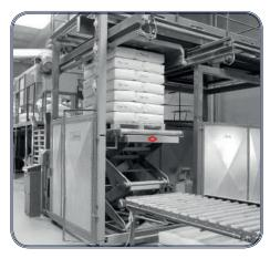
The lifting tables can be constructed for intensive use e.g. in a production line that runs 24-7. The steering can also be made automatic.
